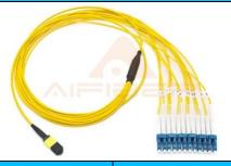
MTP (F) – LC/UPC Breakout cable. MTP 24 core standard connector with 6x LC Duplex connectors. Single-Mode 9/245, G652D, LSZH, 3.0mm cable with each Breakout 2.0mm diameter, with 0.5m length. Standard MTP connector with standard routing and B-Polarity
