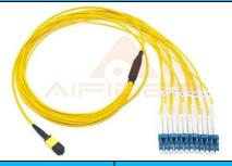
MTP (F) – LC/UPC Breakout cable. MTP 12 standard connector with 6x LC Duplex connectors. Single-Mode 9/125, G652D, LSZH, 3.0mm cable with each Breakout 2.0mm diameter, with 0.5m length. Standard MTP connector with standard routing and B-Polarity
