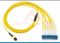
MPO (F) – LC/UPC Fan-out cable. MPO 12 core standard connector with 6x LC Duplex connectors. Single-Mode 9/125, G652D, LSZH, 3.0mm cable with each fan-out 2.0mm diameter, with 0.5m length. Standard MTP connector with standard routing and B-Polarity
