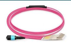
MTP (F) – LC/UPC Breakout cable. MTP 24 core Standard connector with 6x LC Duplex connectors. Multi-Mode 50/245, OM4, LSZH, 3.0mm cable with each Breakout 2.0mm diameter, with 0.5m length. Standard MTP connector with standard routing and B-Polarity
