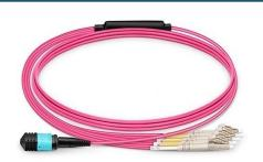
MPO (F) – LC/UPC Fan-out cable. MPO 12 core standard connector with 6x LC Duplex connectors. Multi-Mode 50/125, OM4, LSZH, 3.0mm cable with each fan-out 2.0mm diameter, with 0.5m length. Standard MTP connector with standard routing and B-Polarity
