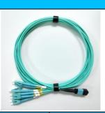
MPO (F) – LC/UPC Fan-out cable. MPO 12 core standard connector with 6x LC Duplex connectors. Multi-Mode 50/125, OM3, LSZH, 3.0mm cable with each fan-out 2.0mm diameter, with 0.5m length. Standard MTP connector with standard routing and B-Polarity
