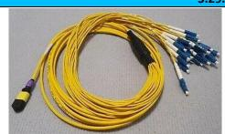
MPO (F) – LC/UPC Fan-out cable. MPO 24 standard connector with 12x LC Duplex connectors. Single-Mode 9/125, G652D, LSZH, 3.0mm cable with each fan-out 2.0mm diameter, with 0.5m length. Standard MTP connector with standard routing and B-Polarity
