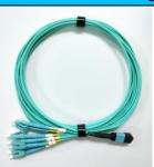
MTP (F) – LC/UPC Breakout cable. MTP 12 core standard connector with 6x LC Duplex connectors. Multi-Mode 50/125, OM3, LSZH, 3.0mm cable with each fan-out 2.0mm diameter, with 0.5m length. Standard MTP connector with standard routing and B-Polarity
