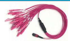
MPO (F) – LC/UPC Fan-out cable. MPO 24 standard connector with 12x LC Duplex connectors. Multi-Mode 50/125, OM4, LSZH, 3.0mm cable with each fan-out 2.0mm diameter, with 0.5m length. Standard MTP connector with standard routing and B-Polarity
