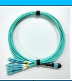
MTP (F) – LC/UPC Breakout cable. MTP 24 core standard connector with 6x LC Duplex connectors. Multi-Mode 50/245, OM3, LSZH, 3.0mm cable with each fan-out 2.0mm diameter, with 0.5m length. Standard MTP connector with standard routing and B-Polarity
