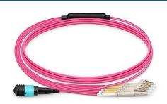
MTP (F) – LC/UPC Breakout cable. MTP 12 core Standard connector with 6x LC Duplex connectors. Multi-Mode 50/125, OM4, LSZH, 3.0mm cable with each Breakout 2.0mm diameter, with 0.5m length. Standard MTP connector with standard routing and B-Polarity
